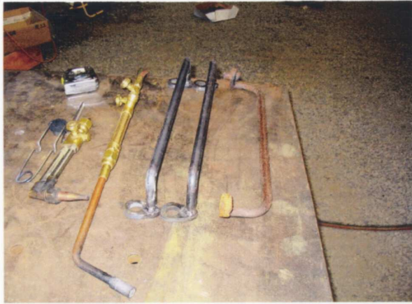
(LEFT) Any grab iron off the P&E hopper car not too badly bent out of shape was heated and pounded straight. We were able to save many of the grab irons in this manner. — Ric Aubin photo
