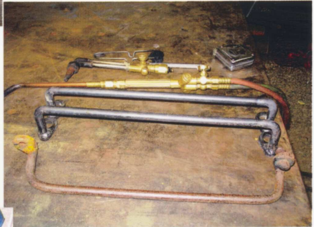
(RIGHT) This photo shows a slightly bent, original grab iron in front of two newly fabricated ones. Medford Fabrication has consistently provided us with their expertise. — Ric Aubin photo
