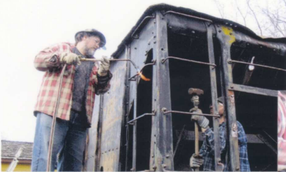
(LEFT) Now it's John Powell's turn to use the torch on one of the rungs. This particular rung only needs a little straightening, so while John heats the rung, Dave applies hammer force from behind. Rick Aubin photo
