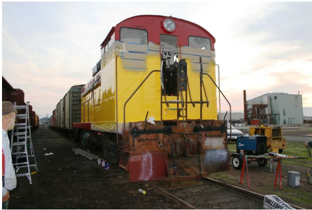
(ABOVE) This view of the cab end shows the red color masked off from the area painted yellow. The end steps will be painted black soon.
