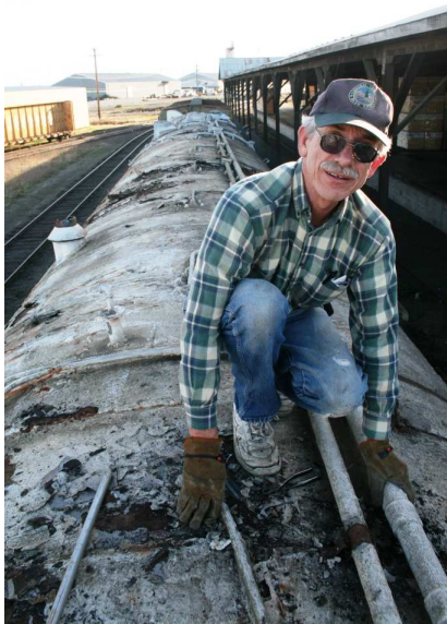
(LEFT) Dan Wilkinson is busy removing dirt and loose roofing materials from around the many holes. He will later begin removing the two long pipes he's kneeling on. These ran the whole length of the car. These were added by SP long after the car was built and therefore will not be needed when we restore the car. (ABOVE) This close-up view shows a large hole near the pipes.
