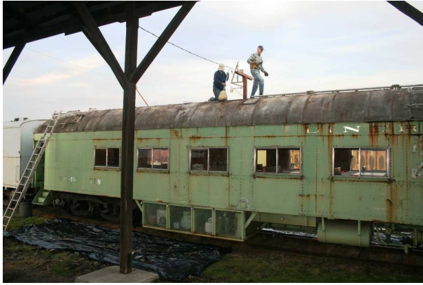
(ABOVE) Dan Wilkinson & Chrisanne Murray are standing on our dining car roof, removing loose material from around holes.
