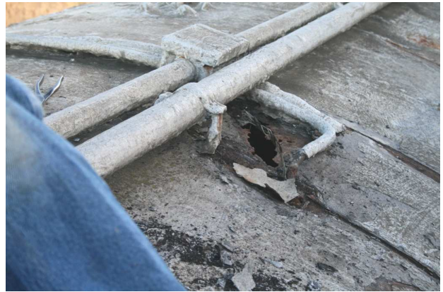
(LEFT) Dan Wilkinson is busy removing dirt and loose roofing materials from around the many holes. He will later begin removing the two long pipes he's kneeling on. These ran the whole length of the car. These were added by SP long after the car was built and therefore will not be needed when we restore the car. (ABOVE) This close-up view shows a large hole near the pipes.
