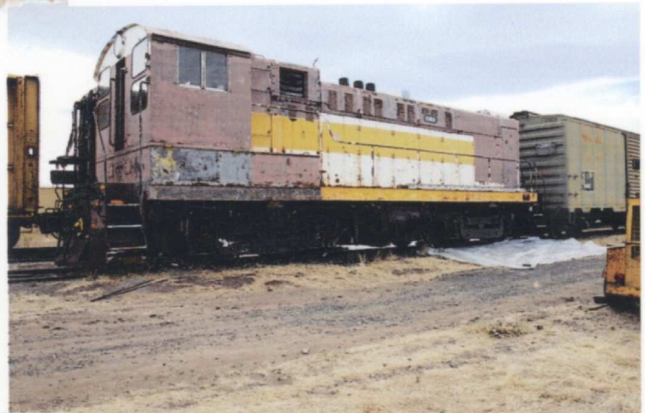
(RIGHT) This is how the engineer's side of No. 8 looked on Oct. 01 after a couple of work sessions. The old paint is gone from the cab, battery boxes, top and end of the hood, and part of the frame. — Tony Johnson photo
