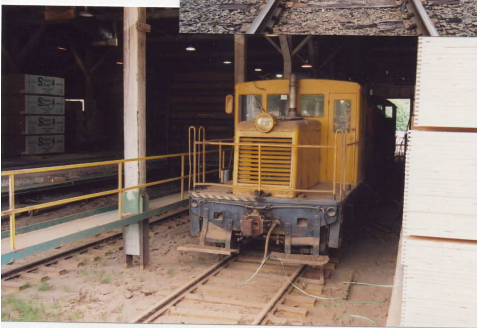
(LEFT) Here is one of the two switchers that belong to Superior Lumber Company. This 45-ton General Electric locomotive was built in 1942 for the U.S. Army. After the war it came to Glendale, Oregon to work for the Robert Dollar Company, and next the Gregory Timber Company before Superior purchased the mill.
