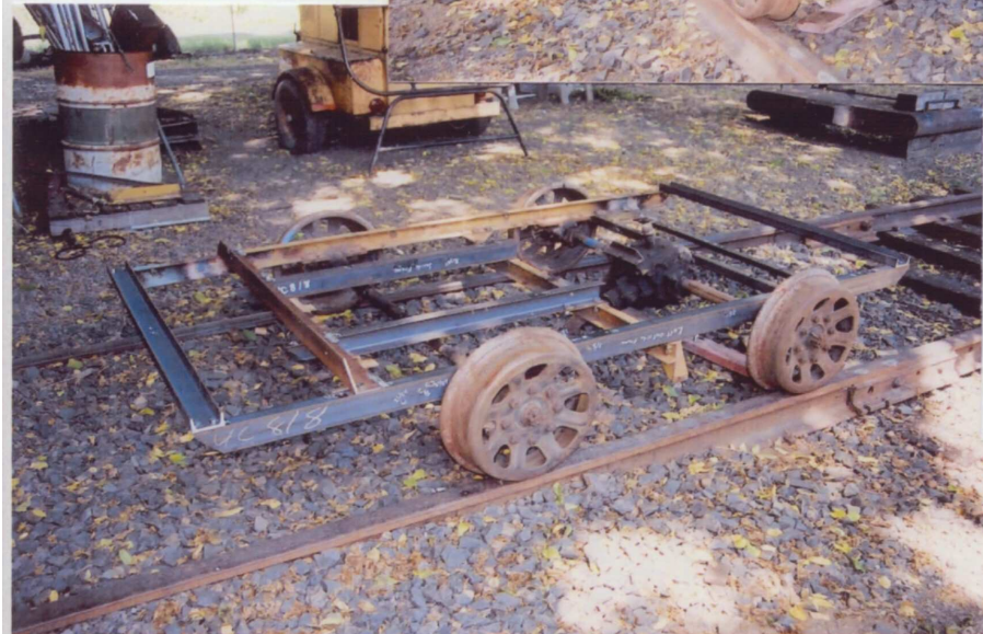
(LEFT) From this angle you see the unpainted sections that represent new frame members fabricated by Jerry. The transmission is in place and soon the engine will be reinstalled. The wood bench seating and covers over the engine will follow after that. We are hoping the A-3 will be running in the park by August.
