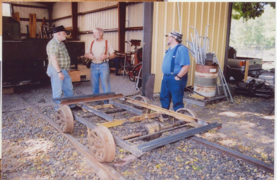
(LEFT) From this angle you see the unpainted sections that represent new frame members fabricated by Jerry. The transmission is in place and soon the engine will be reinstalled. The wood bench seating and covers over the engine will follow after that. We are hoping the A-3 will be running in the park by August.
