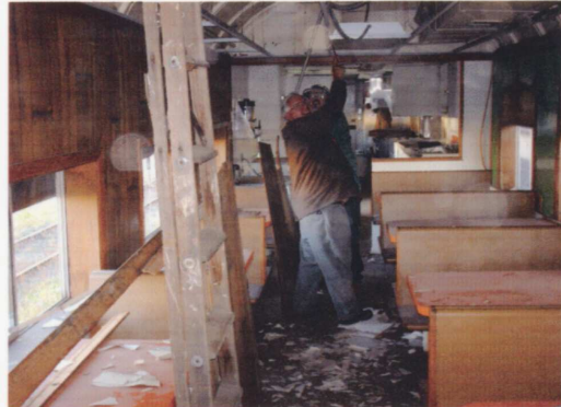
You see here one of the two original ceiling light fixtures applied when Pullman constructed the car for SP subsidiary Texas & New Orleans back in 1912. The two fixtures will be removed for safekeeping as we'll want to find others or have them replicated.—Dan Wilkinson photo
